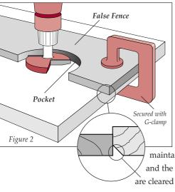
If you are working with an overhead router then the best procedure is to make a false fence in plywood or MDF with a pocket for the cutter to locate – *see fig* 2.
