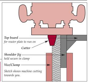
Cutters can be used as above sketch, or inverted in a router table. See Titman Router Table, in our General Catalogue.
