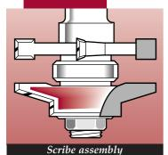
Panel or glass dimensions are determined by the distance between the bottom of the grooves. Allow 2-3mm for correct fit, do not apply glue to the panel as this will restrict any shrinkage and cause the panel to split.
